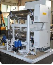
Electrical heaters for heavy fuel, oil and engine cooling fluid
